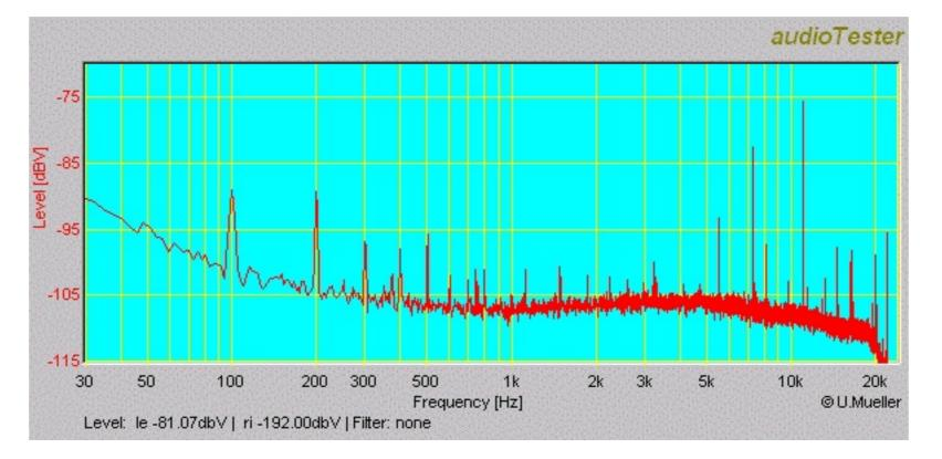
Because we can also hear differences between different brands of CD-Rs playing on the same CD player, we measured the phase comparator output to look at this situation as well. The following picture is from a Philips Premium Silver, where the previou pink noise track has been recorded upon (using a Plextor PX-412 and an Apple Macintosh), played on a CEC CD transport. This resulted in the following figure:
