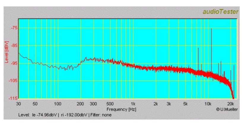
The second figure is from a Micromega player. You can see some lower spectral contents from 200-1000Hz, and there is a spike at 15kHz.
