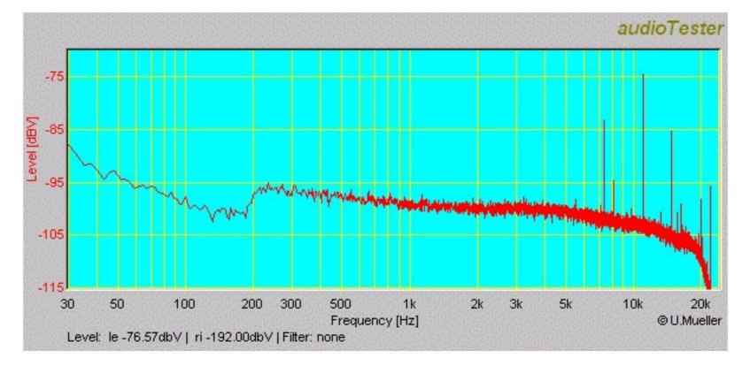
The third figure is from a CEC players. From this figure you can see that the average level of jitter is higher than the former two. You can also se a 100Hz spike, probably due to bad supply rejection.
