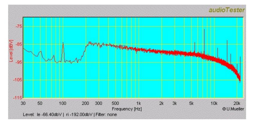
The fourth figure is from a TEAC. There are some spikes at multiples of 50 Hz (supply frequency).
