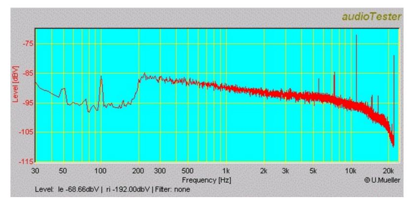
The next picture is the same info, but then at a Ricoh. The measurements have been performed a couple of times, but the spike at 7kHz was a repeatable difference between the two measurements:
